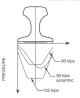
Typical pressure distribution in the transverse direction for a rail on MK6-RFS GANTREX pad.
