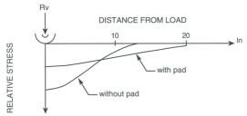
This diagram shows the relative stresses for installations with and without pad.
